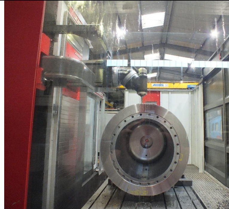
Hydraulic cylinder, piston diameter 710 mm, rod diameter 530 mm, stroke 1250 mm, weight 16200 kg
