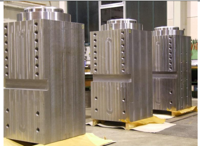
Hydraulic cylinder, piston diameter 675 mm, rod diameter 645 mm, stroke 500 mm, weight 9900 kg
