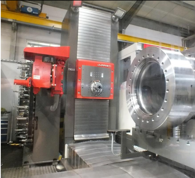
cylinder tube, piston diameter 1300mm, weight 18900 kg
