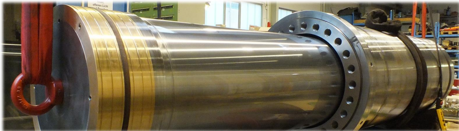
Hydraulic cylinder, piston diameter 780 mm, rod diameter 720 mm, stroke 1000 mm, weight 10900 kg
