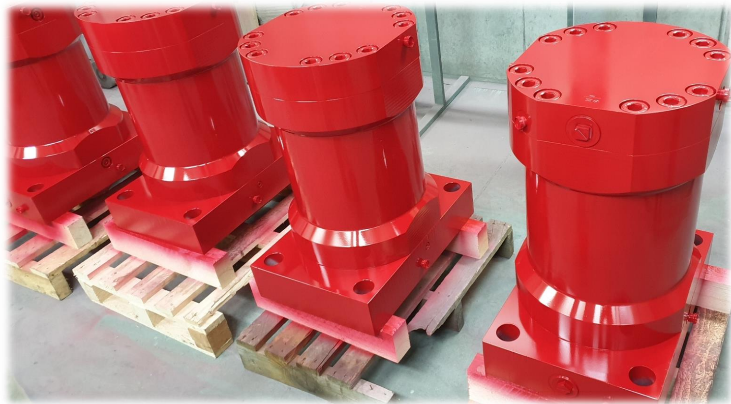
Hydraulic cylinder, piston diameter 305 mm, rod diameter 140 mm, stroke 308 mm, weight 526 kg
